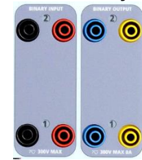
Figure 170 Binary Inputs and Outputs 1 and 2
