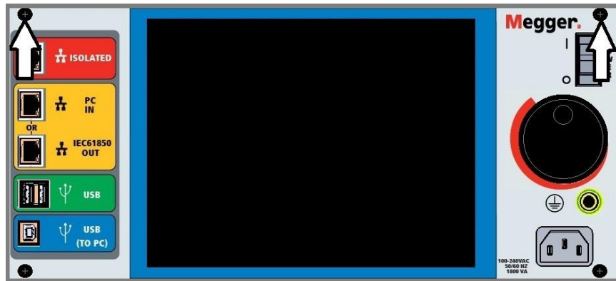
Figure 228 Top Panel Removal Front Panel Screws
