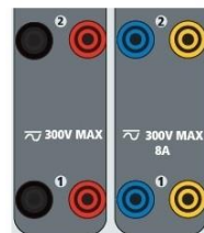
Figure 190 Binary Inputs and Outputs 1 and 2
