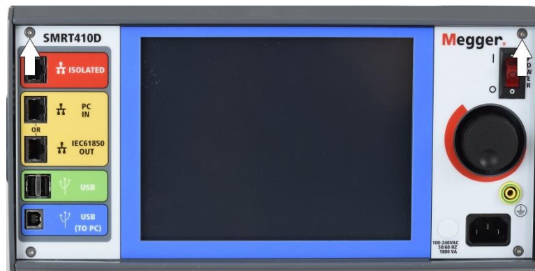
Figure 270 Front Panel Screws, Removal of Top Cover
