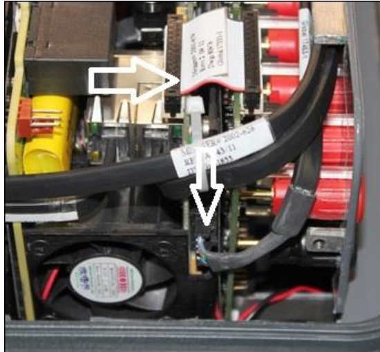
Figure 252 VIGEN1 to Front Panel Cable
