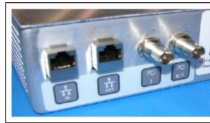
Figure 155 SMRT1 Rack Mount Back Panel Signal and Communication Ports
