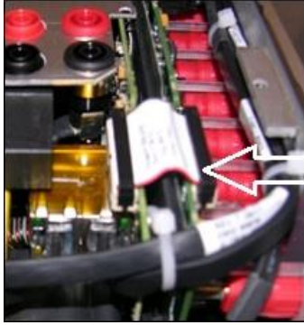
Figure 187 VIGEN1 to Front Panel Cable
