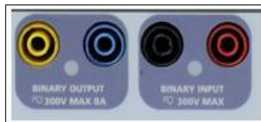
Figure 156 SMRT1 Binary Input and Output
