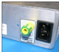
Figure 154 SMRT1 Rack Mount Back Panel Power Input
