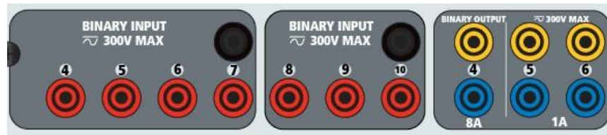
Figure 191 Binary Inputs 4 to 10 and Binary Outputs 4 to 6
