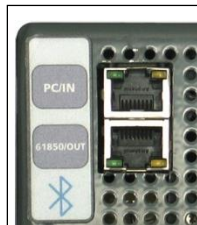
Figure 157 SMRT1 Communication Ports
